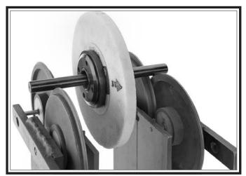
Figure 39. Wheel on balancing fixture.
